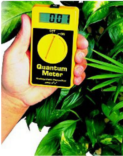
A commercial handheld (photosynthetically active radiation) PAR light sensor (photo Quantum Light Meter).
